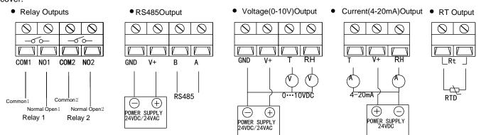
\*Current 4-20mA Output: terminal RH loop should be connected, otherwise the transmitter can not work.
